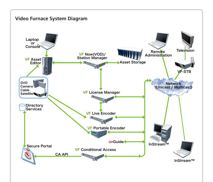
The above diagram highlights the architecture of the Video Furnace solution. From creating, managing and scheduling your own digital assets, to broadcasting live video signals. Support for either Multicast (NVOD) or Unicast (VOD).
